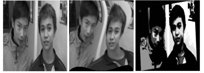
(a) One frame of the original video (b) Frame after random bending (c) Frame after MPEG 4 compression, rotation and random contrast adjustment
